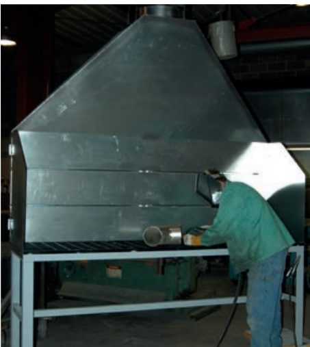
8' SFH with Hinged Side Shields, for Welding Table Application
